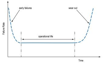
The failure rate is derived from our periodic test results. The failure rate ( $\lambda_R$ ) is, therefore, only given at test temperature for life tests. An estimation is also given at 60°C.
