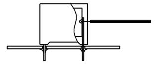
Temperature monitored inside the capacitor.
