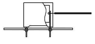
Temperature monitored inside the capacitor.
