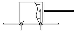
Temperature monitored inside the capacitor.
